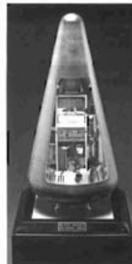
Figure 3 An early Black Knight re-entry head, sectioned for display. This artefact was used at the Royal Aircraft Establishment for research and instruction during and after the Black Knight programme. (Science & Society Picture Library)
