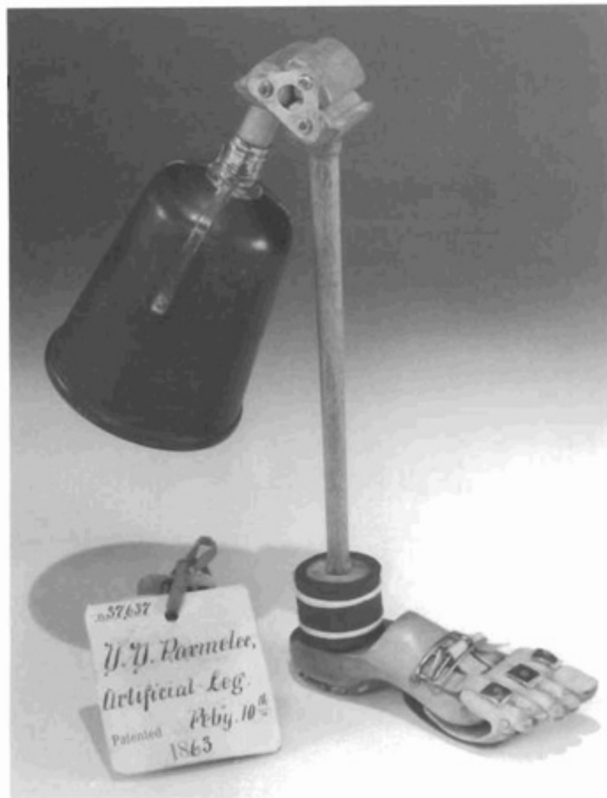
Figure 1 This 1863 prototype leg was submitted by D D Parmelee along with his patent application. The innovation points in nineteenth-century artificial legs were flexion (ankle and knee joints) and attachment. This leg has an ingenious knee design and a complicated toe attachment. (Collections of the Division of Medicine and Science, National Museum of American History, Smithsonian Institution)
