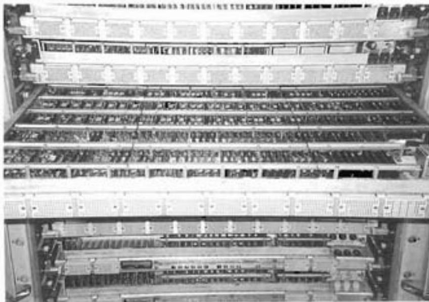
Figure 2. Close-up of the NTDS Circuits. The dense packing of the individual circuits was an indication that Seymour Cray was involved. The NTDS used discrete transistors, not integrated circuits.
