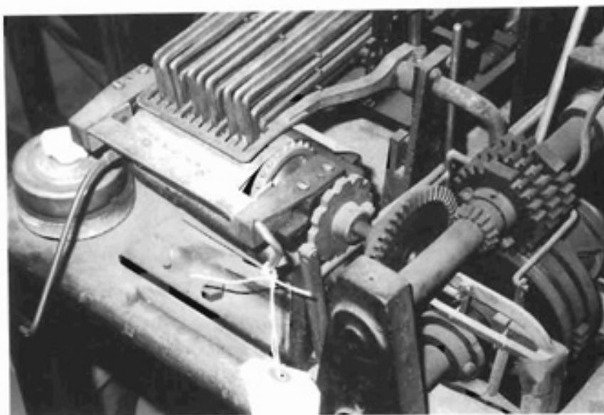
Figure 7. The detail shows arrangement of the reading fingers. One can see the massive design of the parts of the machine, which is stronger than any recent calculating machines. (Photo taken by H. Petzold, 1997.)
