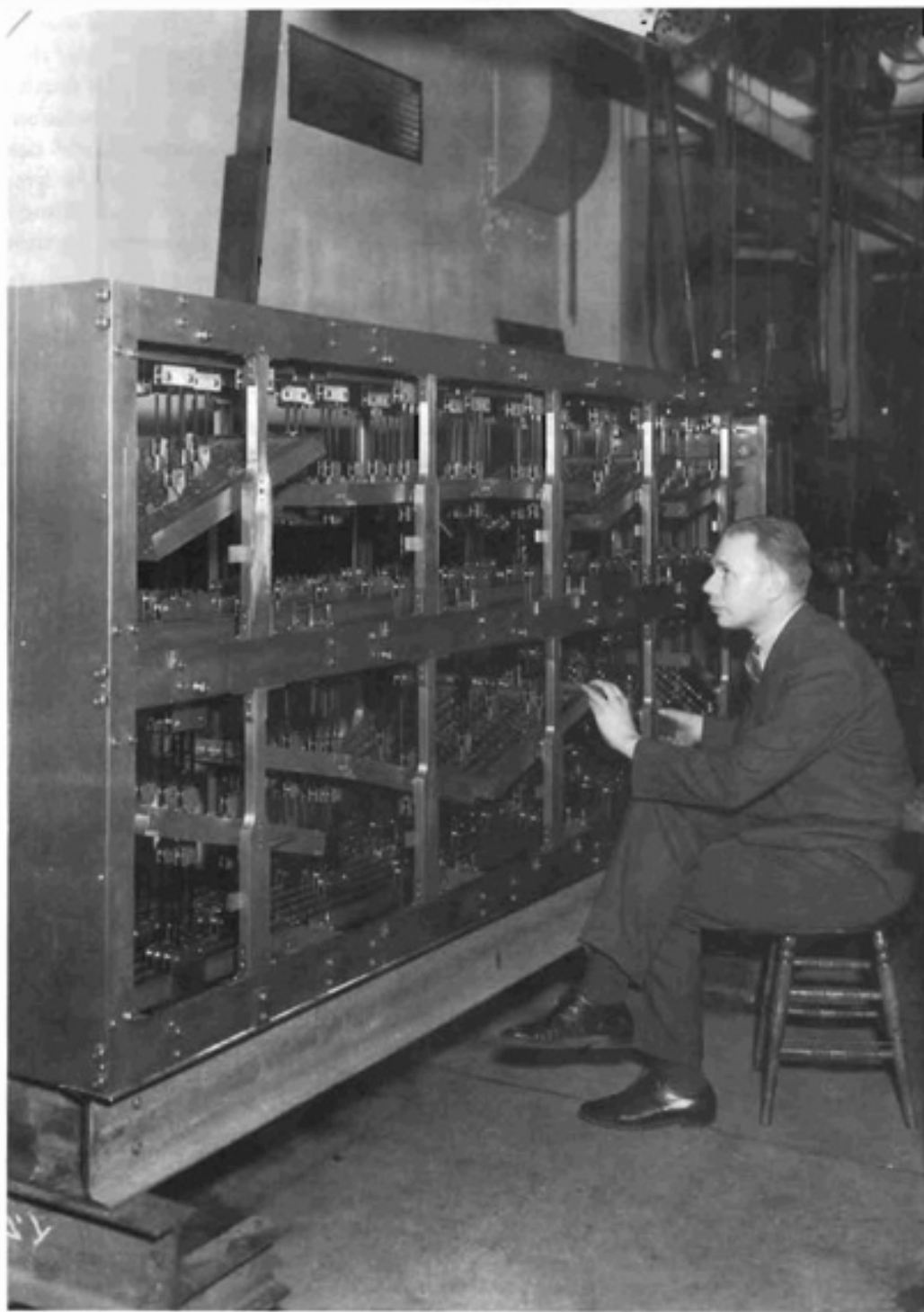
Figure 11. Wilbur sitting before the Simultaneous Equation Solver, setting a coefficient. (Photo MIT Museum)
